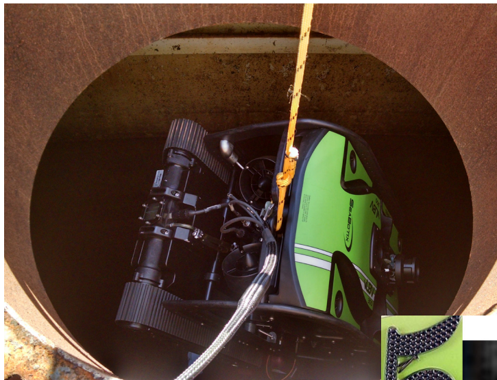
Storage Tank Surveyor being lowered thru tank manway.
